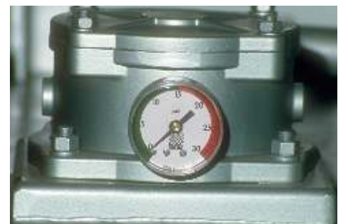
To simplify maintenance, the power unit features a filter gauge to indicate when the filter should be changed.
