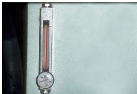
Sight glass indicates the hydraulic oil level and temperature.
