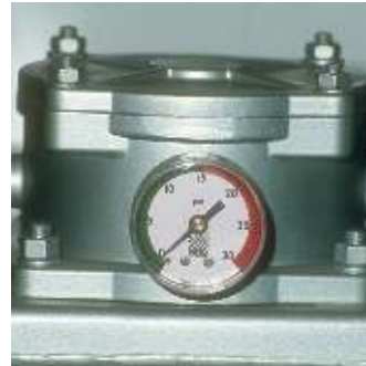
To simplify maintenance, the power unit features a filter gauge to indicate when the filter should be changed.
