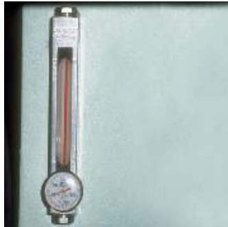
Sight glass indicates the hydraulic oil level and temperature.
