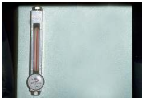
Sight glass indicates the hydraulic oil level and temperature.
