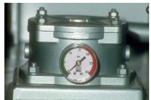
Convenient, easy-to-read gauge indicates when oil filter needs service.
